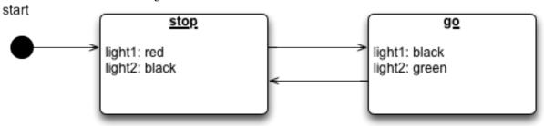
When the system is switched on it goes automatically into the stop mode as default state. The stop state changes the light1 to red and light2 to black (off). An external event can trigger now a state switch to the "go" state. In the go state we change the color properties from light1 to black (off) and light2 to green to indicate the passers may walk now.
